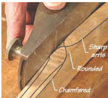
▲ Pic.2 I used a block plane to form an arch-shaped arris
